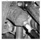
4. Once you have cut the bands pull the boot down to expose the end.
