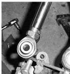
14. Using a ½" drill bit or equivalent, open the hole of the knuckle assemble to ½".
