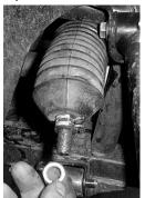
11. Connect the rod to the rack and pinion with the small tapered end connecting to the left hand heim.
