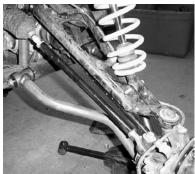
2. Disconnect the rod from the knuckle assembly.
