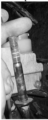
10) Now place the Small Spacer onto the rod and place the rubber bumper back on the rod and connect the stabilizer bar to the stabilizer rod.
