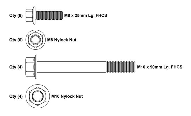
Do not tighten hardware completely unless noted. Keep all components removed from machine.
