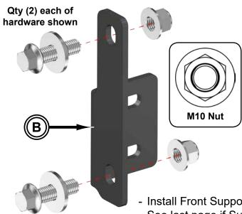
Install Front Supports (B)(C) with hardware shown.
