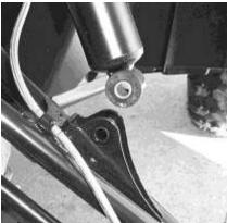
4) Disconnect the bolt securing the brake line near the shock mount. You will need to use zip ties provided to secure the brake line once the lift kit is installed.
