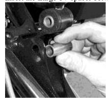
6) Connect the front lift mounting bracket to the A-arm by using a 10x70 bolt. Slide the bolt thru the bracket and spacer between the shock mount tabs.
