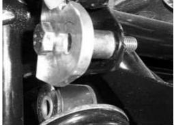
12) Place the second lift bracket into place next to the shock mount making sure that it nests against the shock mount tab.
