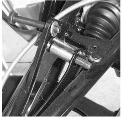
8) Push the 10x70 bolt thru placing another 10mm washer on the opposite side of the shock eyelet. Connect it all together using another front lift bracket and 10mm locking nuts.
