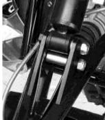
9) Use the zip ties provided to secure the brake line to the control arm.
