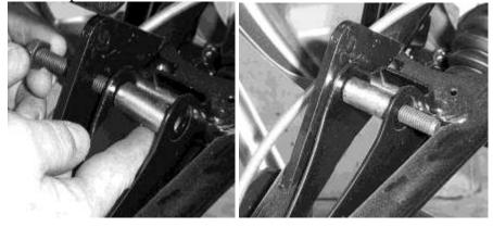
7) Next insert a 10x70 bolt thru the top of the lift bracket, and then place a 10mm washer on the bolt.
