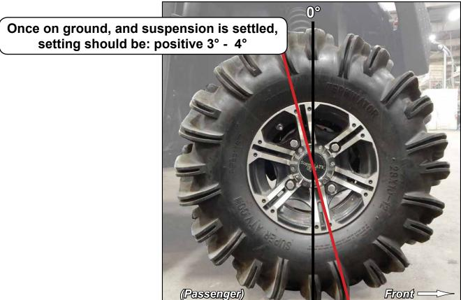
Adjust Pivot Blocks, in or out, to achieve correct setting. One Pivot Block will be different.
