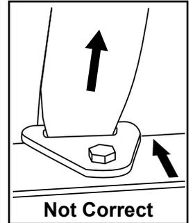
Mounting Brackets are to be installed at an angle that is the same as the direction of pull. Preferred mounting is as shown above. Ensure there are no welds around Belt or Belt Hardware. All mounting points are to be directly to frame of vehicle chassis. Belts are to be mounted so that drivers forward and upward movement are limited.
