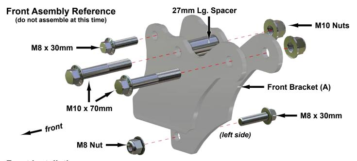
Front installation: Do not tighten hardware completely unless noted.
