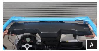
A. With one person on either side of the vehicle place the WP-CM04 into location from the underside of the cage.
