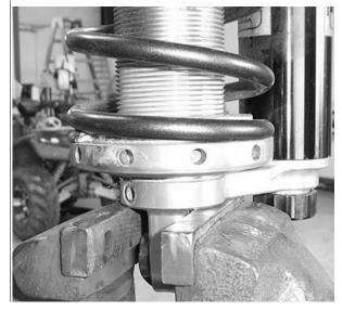
3. Compress the spring and remove the retaining collar from the shock.
