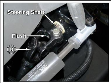
Upper Shaft and Steering Shaft Adjustment:
