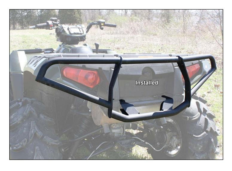
Do not tighten hardware completely unless noted. Keep all components removed from machine. Components (A) through (D) may be put together prior to installing on machine. Following instructions are for assembling Bumper, in sections, to machine.
