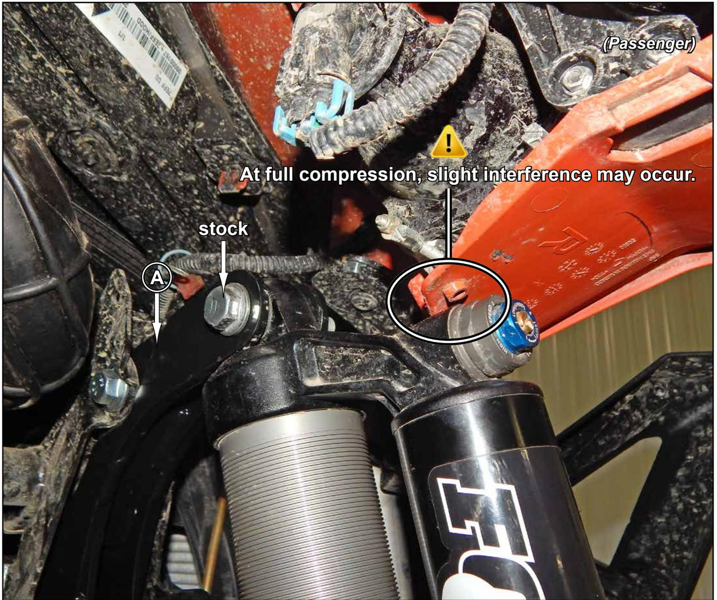
**Rear Removal:** *Keep all components removed from machine.*
