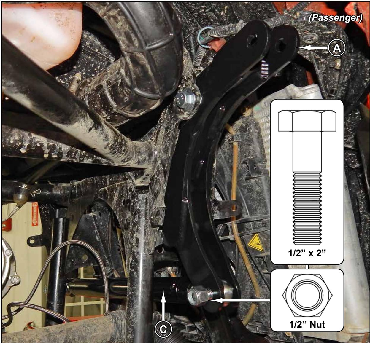
**Tighten hardware completely.**
