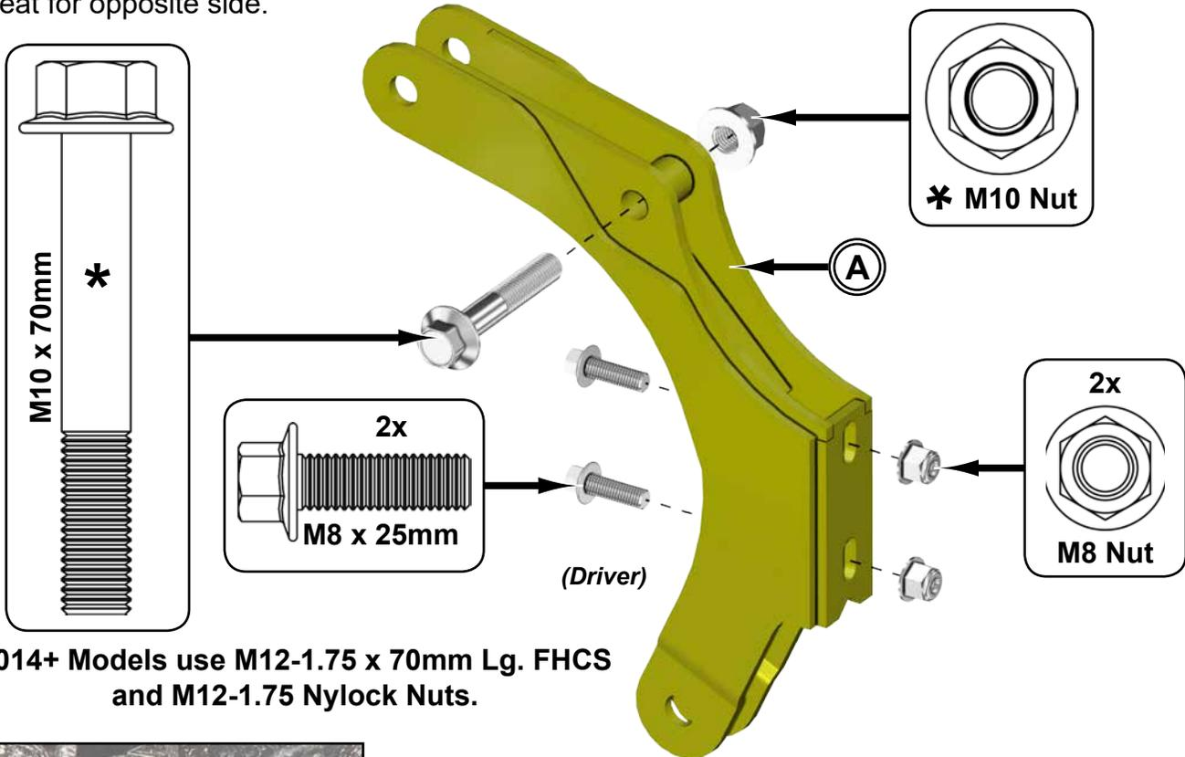
\* 2014+ Models use M12-1.75 x 70mm Lg. FHCS and M12-1.75 Nylock Nuts.
