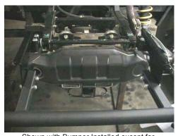
Shown with Bumper Installed except for 5/16" Self Tap & Bed Removed.
