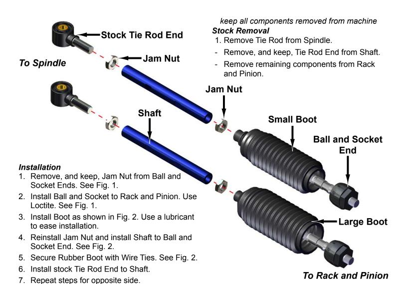
(Rack and Pinion shown off machine for clarity)
