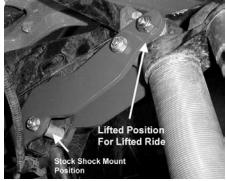
Rotate the piggyback reservoir on the shock 180 degrees. Rotates very easy by hand.
