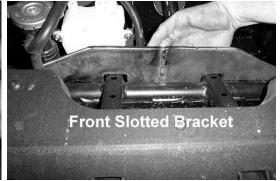
5. Place spacer between the shock mount tabs and insert the 10mm x 65mm hex bolt through the slotted bracket and spacer.
