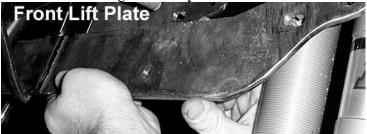
7. Now secure the plates loosely with the 10mm lock nut.
