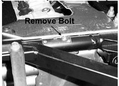
7. Disconnect the top of the rear shock from the shock tabs.
