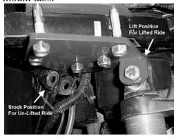
3. Once you have moved the shock torque all nuts and lower the jack.
