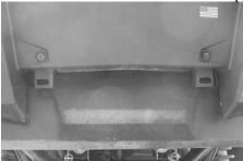
2. Using the two ¼ x ¾ button head bolts, ¼" washers and ¼" lock nuts connect the plate to the license plate location.
