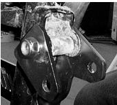
5) Then connect the top of the shock to the lift brackets, placing one 10mm flat washers between the shock and brackets, securing it with a 10x65mm bolt. Secure it with the 10mm lock nut.
