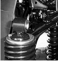
4) Slide the long front lift bracket next to the frame. It should run from one shock mount to the other, on the front side.
