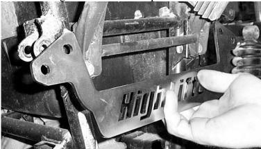
4) Place the spacer in the shock mount and the small lift bracket to the rear of the frame holding it in place with the 10x65mm bolt and fasten with 10mm lock nut.
