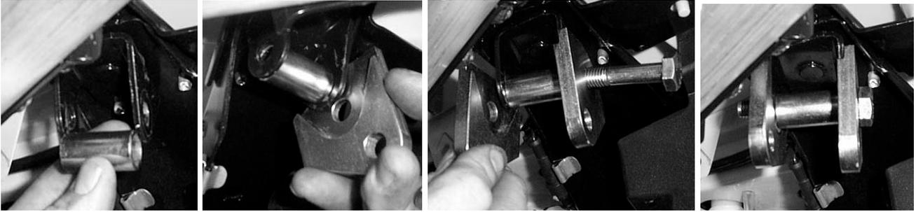
NOTE: If the brackets do not fit just right the Stock Shock Mount is Adjustable and can be moved. You may need to adjust it to make the brackets fit properly.
