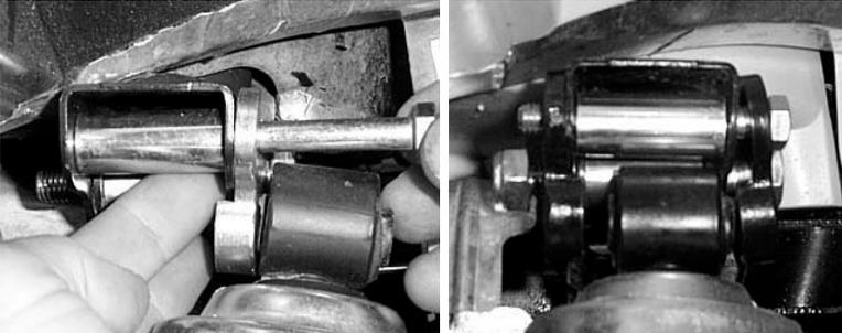
8. Connect the top of the shock between the two lift brackets using a 10x65 hex bolt and 10mm lock nut.
