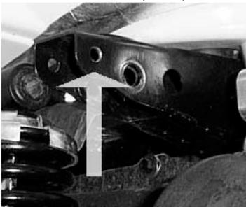
5. Insert one 10x 65mm hex bolt thru one of the right lift brackets, and then place the small rear spacer into the stock shock mount location. Insert the bolt thru the shock mount and spacer.
