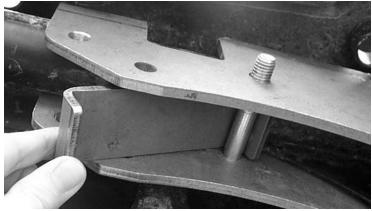
12. Push the rear lift plate all the way up touching the frame and insert a 12x70mm hex bolt.
