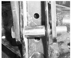
10. Next you need to attach the rear lift plate. Insert a 12x70mm hex bolt through the bracket.
