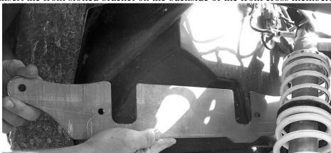
11. Connect the bracket to the frame by placing it on the bolts and fasten it using the 10mm lock nuts provided.
