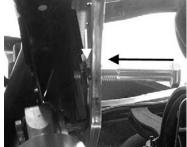
9. Next insert a large spacer in the stock shock mount position and push the 10x70mm bolt through. Repeat steps for the opposite side at this time.
