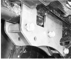
14. Now connect the top of the shock to the lift brackets by inserting another 12x70mm bolt through the bracket. Insert the rear shock spacer between the shock eyelet and bracket.
