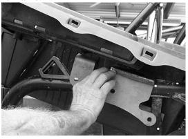
7. Once you have the bracket in place connect it to the stock shock mounting tabs using the 12x70mm bolt and 12mm washer provided in the kit. Make sure that you insert the 12mm washer between the shock mounting tab and the bracket.
