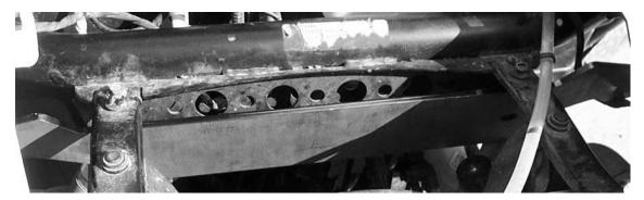
8. Insert the 10 x 70mm bolt through the bracket, placing a 10mm washer between the bracket and the shock mount.
