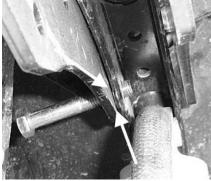
8. Next, place a spacer where between the shock mount tabs. Then, insert another 12mm washer between the shock tab and the bracket.
