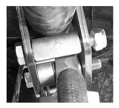
15. Fasten tight using a 12mm lock nut.
