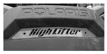
4. Using the two 5/16 x 1" button head bolts, 5/16" washers and 5/16" lock nuts connect the plate.
