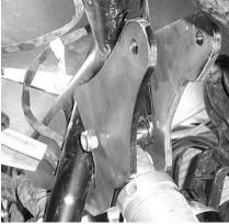
12. Connect the top of the shock to the lift plates. Insert the 10 x 70mm hex bolt through from the backside forward. Place a small front shock spacer between the shock eyelet and the lift plate. Fasten it tight using a 10mm lock nut provided.
