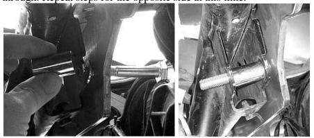
10. Insert the front slotted bracket on the backside of the front cross member.
