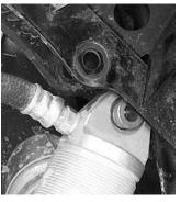
6. Now that you have disconnected the top of the shock from the frame, you will need to insert the rear lift bracket through the plastic onto the frame.
