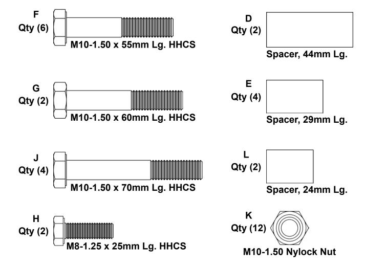
Do not tighten hardware completely unless noted. Keep all components removed from machine.
