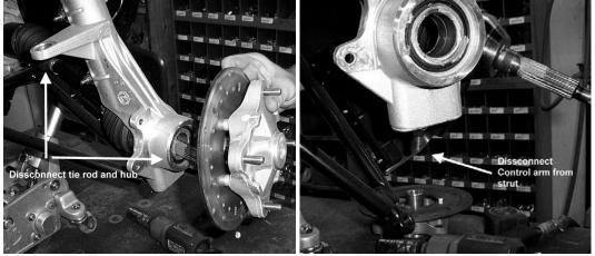
4) There are two ways you can install the lift. You can take the strut and springs completely off. If you do this, then the front plastic will need to come off on the newer models. We are going to show you a "short cut" method.
